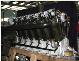
Right side view showing exhaust attachment and (E1) detail.
