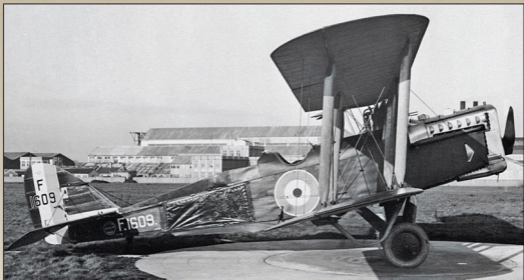
Westland built DH.9a F1609 from page 10. Note the unpainted aluminium engine cowlings with black hinge detail and that no Scarff ring or gun sights are fitted.
