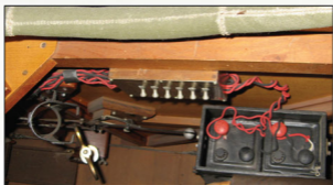
Observer's throttle (A5), seat and Lewis gun ammunition drums (A2). Note the interior colour of the linen fuselage covering.
