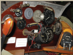
Instrument board detail from F1010 after full restoration. Note the placement of decal 70 behind the compass and 92 & 93.
