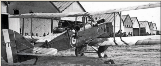
Before... AMC built DH.9a H72 seen here in service with 27 Sqn in 1922 where it has been turned into an airmail furniture delivery vehicle. In addition to the bed and suitcase strapped to the rear of the fuselage there are bundles of stores slung from the wing bomb carriers. Note the starboard bottom wing cut out has been extended and the engine side cowlings have been removed.
