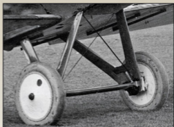
Undercarriage detail from Westland built DH.9a H3452. The metal brackets appear to be painted black p . Palmer Cord Aero wheel cover markings 40 are faintly visible.
