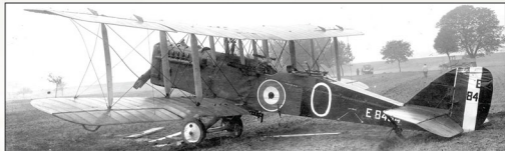
This AMC built DH.9a E8484 was one of seven 110 Sqn aircraft to be lost (out of a total of 12) when they failed to return from a bombing raid on Frankfurt on 21 October 1918. E8484 had been on squadron strength for just 4 days and the crew of 2Lt A.W.R. Evans and Lt R.W.L. Thompson were both made POW. Note the damage to the propeller, port wing and rudder from when it overturned on crash landing and how dark the battleship grey ply areas of the fuselage appear under the overcast sky. AMC company decals [56] can be seen on all struts.
