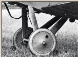
Undercarriage detail from Mann built DH.9a E9703 showing Palmer Cord Aero Tyre markings 42 on 'grey wall' tyres.
