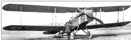
AMC built DH.9a E8483 arrived at 99 Sqn IAF RAF in France on 21 October 1918. This photo was most likely taken after the armistice when many of these great aircraft were relegated to the peaceful duty of carrying mail (see the bags on the ground). It is fitted with a single Carrier 112lb Single Mark II under the fuselage while the Cooper bomb carriers have been removed from under the wings. Note how the starboard bottom wing cowlade does not line up with the aileron indicating a recent replacement and that the white(?) paint is wearing off the wheel covers. The undercarriage legs could be natural wood r or painted i as illustrated. Another photo of E8483 appears on page 29.
