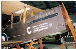
F1Q10 displays its radiator cowling (D13), modified exhaust (D24) and triangular side fairing (D13). Westland Aircraft Works decals (62) have been applied to all struts and undercarriage legs. (David Frowen)
