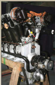
Rear view showing water pump details.
