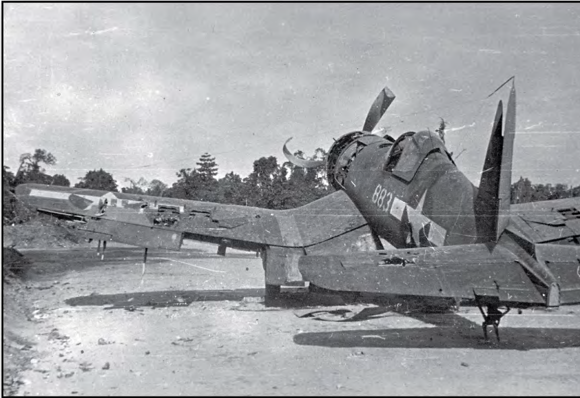
883 in the dump at Vella Lavella in January 1944. Despite the poor condition of the print, several interesting items are visible. First, note the wire antenna. It extends from the insulator lead-in on the right side behind the canopy, up to the rubber insulator attached to the tip of the rudder, then out to a small vertical mast affixed to the root end of the pitot tube (see antenna detail page). Another is the lighter colored border on the upper wing insignia. This has often been interpreted as red, but we disagree. See details on page XXXX.
