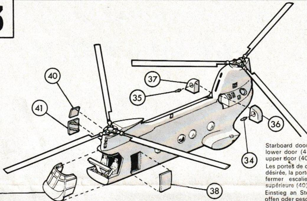
Starboard doors, if open position is desired, lower door (41) drops to form steps; omit upper door (40).
