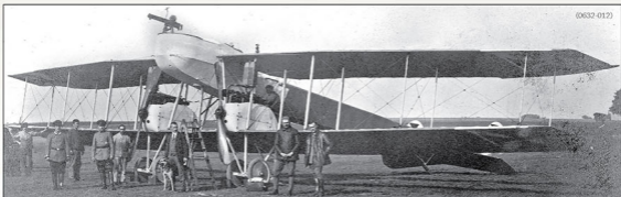
Gotha G.1 9/15 was the production prototype and first aircraft completed from the initial production order and is seen here at Fliegerersatz Abteilung 7 (FEA 7) in Koln in mid 1915. Note the twin core radiators, bomb dropping cage and IMG 08 "Spandau" armament. Although 9/15 was powered by 160hp Daimler-Mercedes engines like UWD 120, the remaining G.1 from the 1st and all 2nd production orders had 150hp Benz Bz.III engines.
