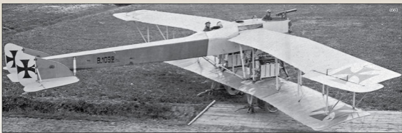
The original Oskar Ursinus designed Friedel-Ursinus Kampfflugzeug "FU" B1092/14 photographed in early 1915 in modified form with balanced ailerons and Hazet radiators to cool its 100hp Daimler-Mercedes D.1 engines. The unequal span wings, angled outer struts and tailplane are the most identifiable differences between this and the Gotha G.1.
