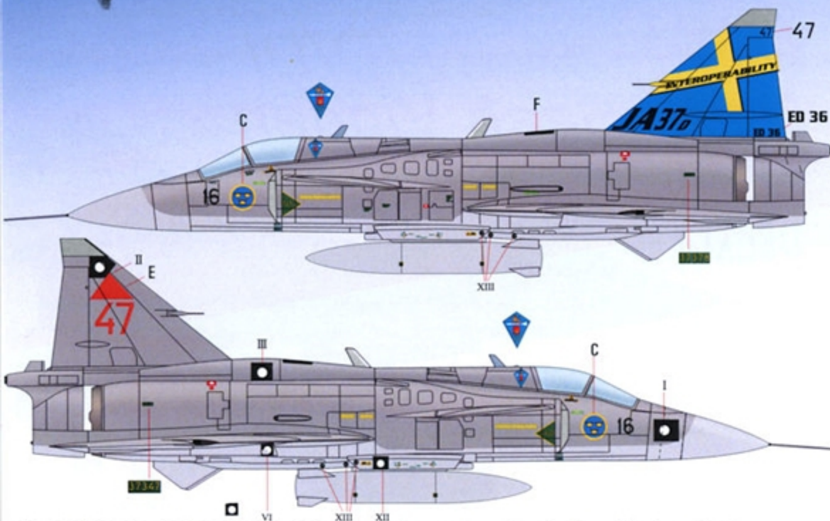
JA 37Di, 37347, 47- FC 2002. This airframe served as prototype for the Di modification. ED 36 indicates the Edit 36 software. The black/white dot-markings on the right side are test validation markings. The modification included capability to carry the Rb 99 AMRAMM Air to Air missiles. Later the F16 wing numbers were removed and an orange band applied around the nose (300 mm wide and black dashed in this view) indicated that the a/c was operated by the FC (Försökscentralen - The Test Establishment).
