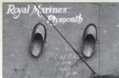
Carburettor intake pipes (E2 + P10) from the unidentified presentation DH.9 on page 7.
