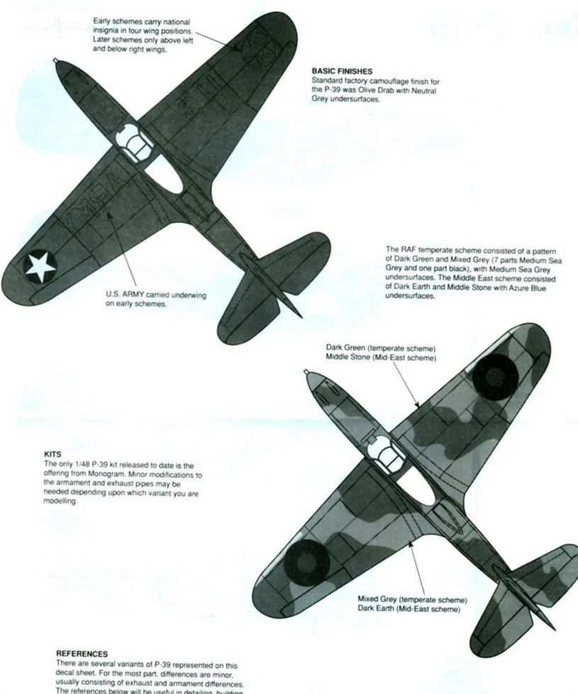
The references below will be useful in detailing, building and finishing the aircraft depicted here.
