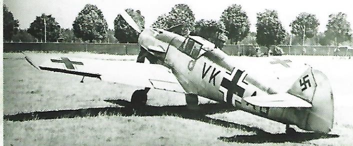
Bf 109 F-0 WNr. 5604 VK+AB. The aircraft with the DB 601 A engine already had the compressor intake with a circular cross-section. It was used to test the newly designed glycol cooler flaps combined with landing flaps. The wing still had the straight ends of the Bf 109E.
