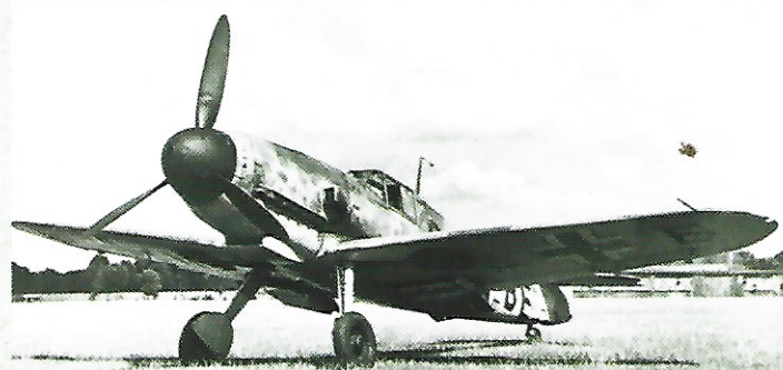
Bf 109 F-0 PH+BE already had oval wingtips, but the intake turbocharger had a rectangular cross-section, characteristic of the Bf 109 F-1 produced by the WNF factory.
