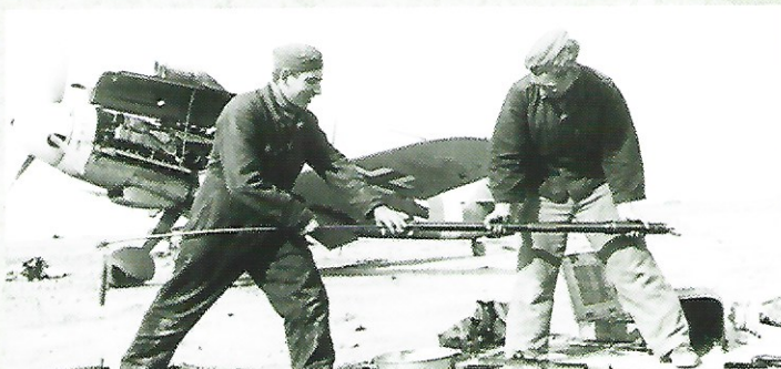
JG 27 Bf 109 F-4 Trop in North Africa. Mechanics are cleaning the barrel of the MG 151/20 cannon.
