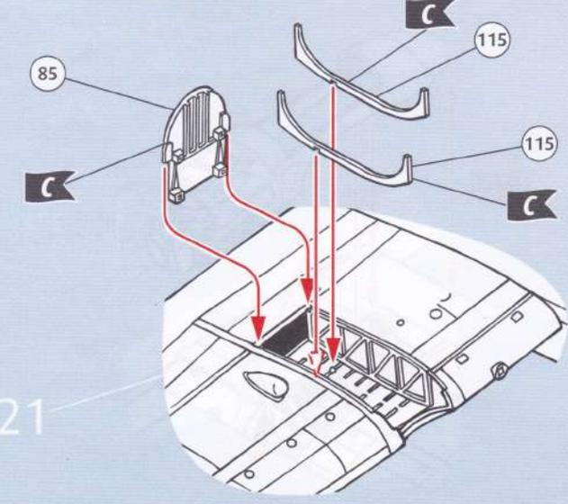
Diagram 22 shows the assembly of a curved component (115) into a larger assembly (21). Red arrows indicate the assembly path.
