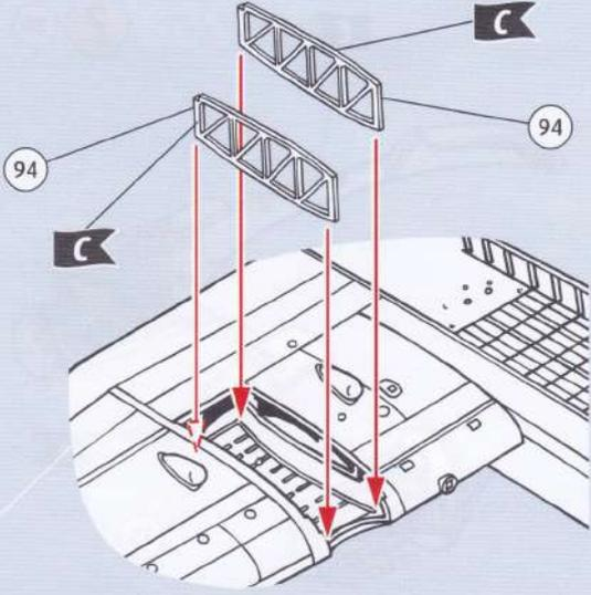
Diagram 21 shows the assembly of a rectangular component (94) into a larger assembly (16). Red arrows indicate the assembly path.
