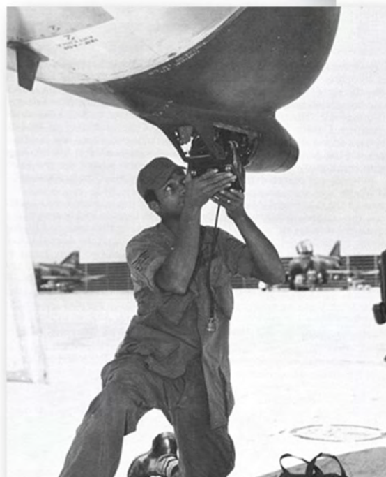
Another view showing an airman loading the aft-facing strike camera in the unique F-4C strike camera radome.
