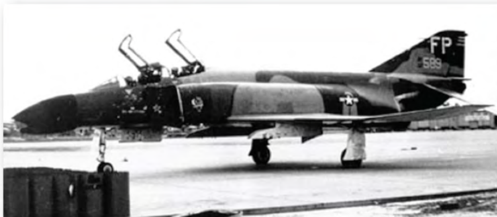
63-7589 taxis in post-mission sometime in late 1967. Note the lack of AIM-9 launcher rails when air-to-ground ordnance was carried
