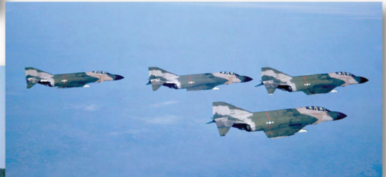
Some examples of the McDonnell factory applied camouflage seen on 64-0927. Both the colors and the pattern by McAir were non-standard. Also note the borderless national insignias on the fuselage (and upper wing), the full turbine warning stripe, and the Futura font style warning placards around the nose. The belly was in the correct FS 36622 on these aircraft.
