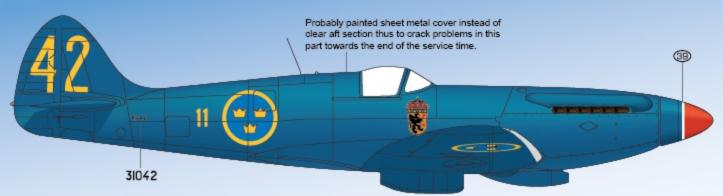
**S 31, 31042, 42 – F11.** During the last years, the Spitfires got the later, more elaborate Coat of arms with gold as later used on the Vampires and Tunnans. The markings are according to the time of an accident when the a/c crashed into an S 14 Fieseler Storch. Pointed blade type, drawing number 10130, decals (24a) and use four decals (51c) plus (51a) or (51b) on the master blade. No Rotol logotype on blades.
