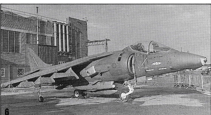
on the starboard side.) Photo: P J Cooper. 6. Sister GR5, ZD347/'04', was statically displayed at Abingdon's Battle of Britain show, 15-16/9/89. Even a quick glance at the GR5 will reveal that it has several external differences to the AV-88, most noticeably the nose profile and addition of the AIM-9 Sidewinder wing pylons. Note the fitment of twin 25mm Aden cannon pods, the centreline store often comprising a baggage pod; the GR5 does not carry the GR3 recce pod. Photo: PJC
